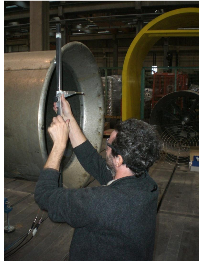
Multi-axial hot-wire measurements on the fan
